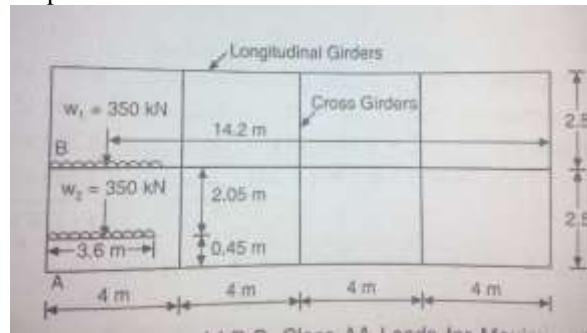
Fig 3.4 Position of IRC CLASS AA TRACKED Load for Maximum Shear
